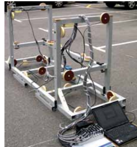
Figure 2. Frame of 27 search coils each having a diameter of 100 mm, and 2000 turns of copper wire
