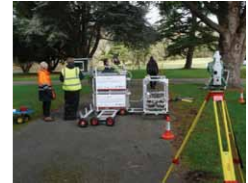
Figure 2. Determining the position of the MTU Mobile Laboratory using an automatic total station
