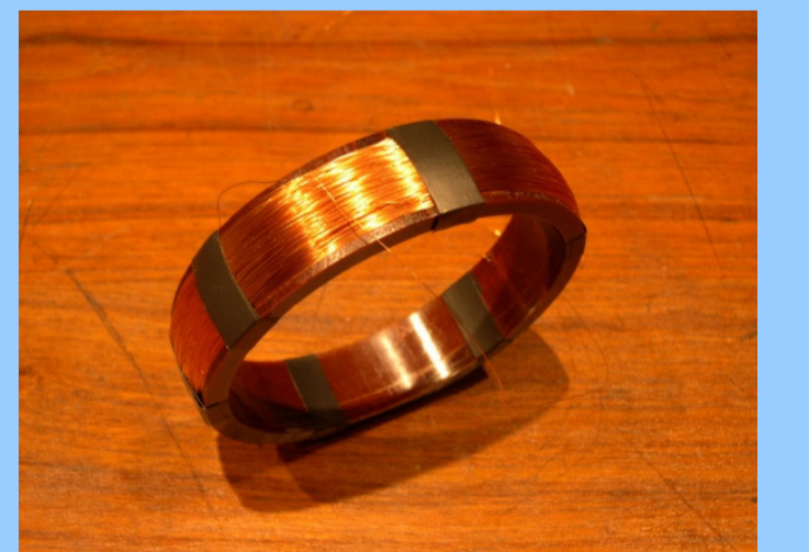
Figure 9: An induction coil designed for this experiment
